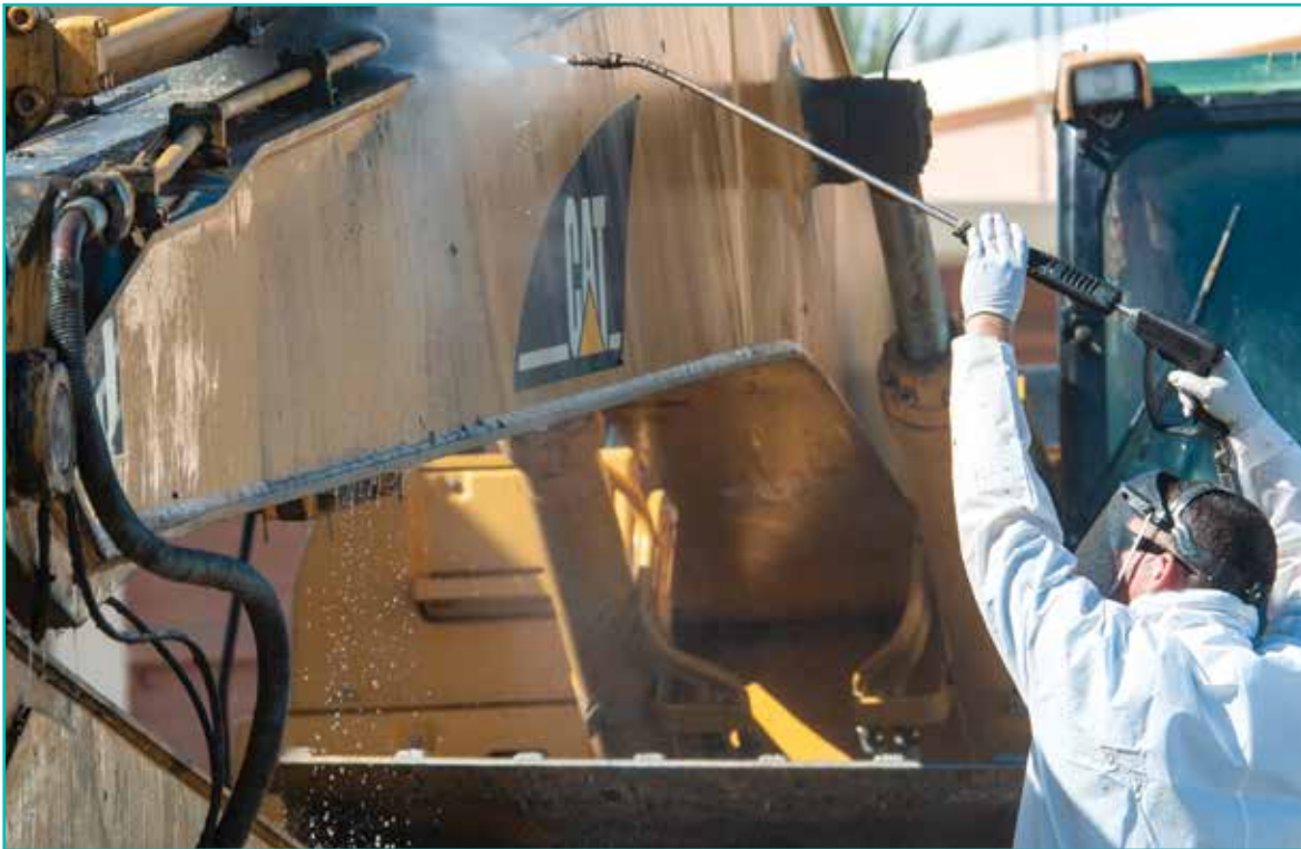
Steam cleaning the arm of a hydraulic excavator
